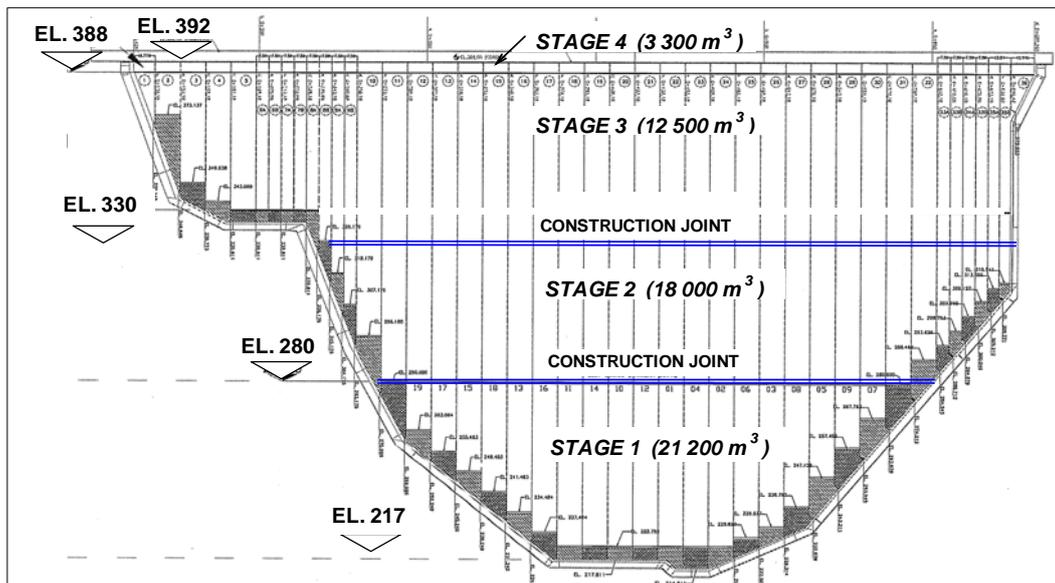
Figure 3. Slipforming stages for the concrete face and approximate concrete volumes.
