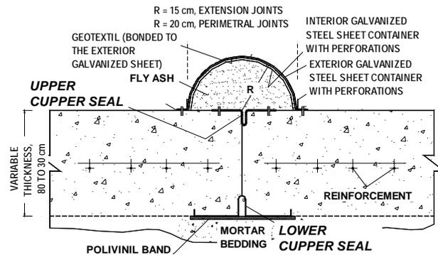
Figure 5. Rolling machine for manufacturing the copper seals, and detail of an extension joint.
