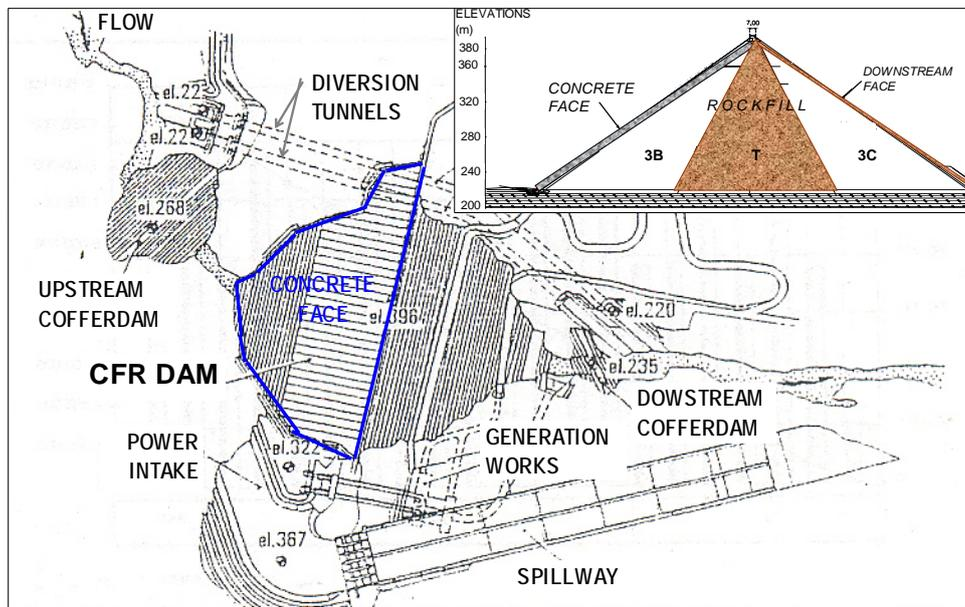
Figure 2. Layout of the scheme and cross section of the dam.
